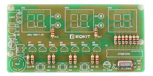
Step 5:Install 1pcs DIP-20 IC Socket at U1. Pay attention to the installation direction.
